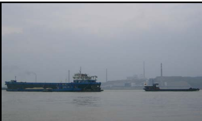
Fig. 7. Two similar barges with (left) and without (right) a full load of sands.
