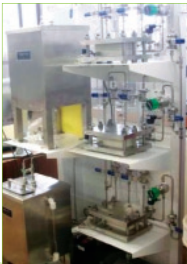
Membranes testing system
